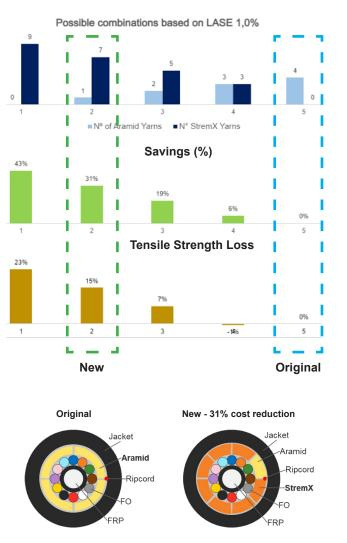
StremX is an inorganic fiber with comparable thermal properties to glass. In addition, StremX presents excellent Processability with current cable production equipment, has superior Fire Resistance, is All-Dielectric, UV resistant and Rodent-Proof
