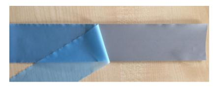
2. <u>Step 2</u>: Place the heat transfer on the substrate surface with the adhesive side down, facing the substrate. For heat press, the temperature and pressure should be even on the tape. Use a press cloth, a siliconized slip-sheet or a Teflon heat pressing sheet to cover the heat transfer and the fabric during lamination to avoid any surface damage. For two times pressing, allow the fabric to cool down after first pressing and press again using the same lamination conditions.
